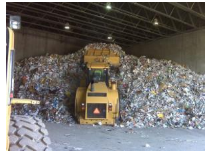
Figure 17. A picture showing the operation of compactor tractors periodically to reduce the volume of waste (Guion, 2025).
