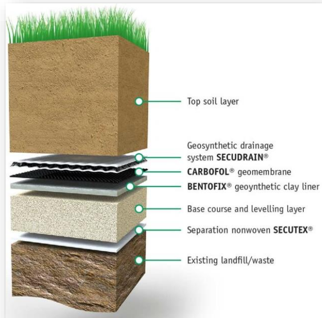
Figure 19. Diagram of final landfill cell cover (Naue, 2025).
