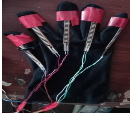
Figure 2: Five flex sensors installed on each finger.
