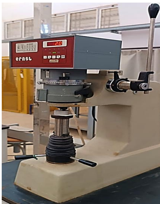
Figure 5: Rockwell hardness tester machine.
